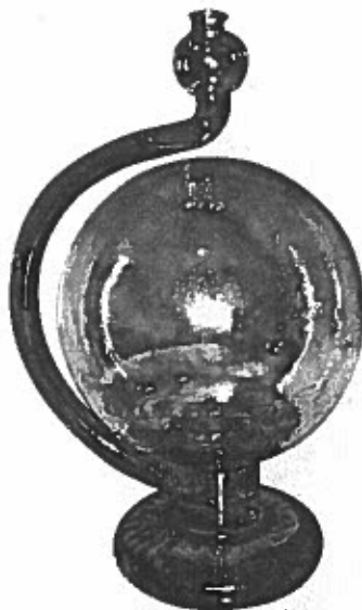
The Storm Glass, the oldest barometer in the world, forecasts changes in weather hours in advance. During high pressure systems (fine weather) the water/food colouring liquid in the glass sits low in the spout; during low pressure systems (storms) the liquid rises, and sometimes spurts out of the spout.
